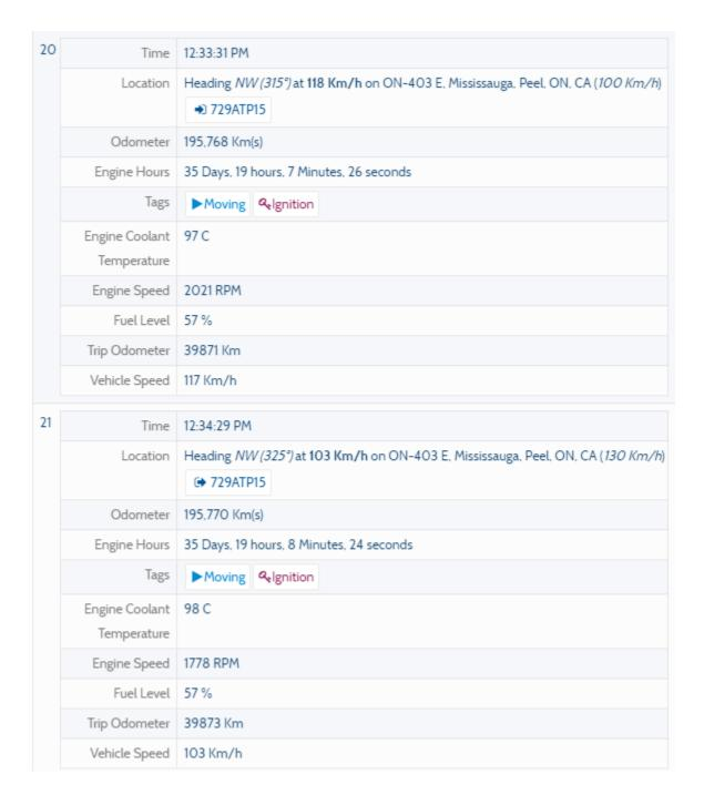
Full Event History - Pull up a complete history for a particular asset; includes time and location event occurred, odometer, engine hours, speed, engine information (if applicable) and Tags (moving, speeding, stopped ignition etc). Report Breakdown example below:
