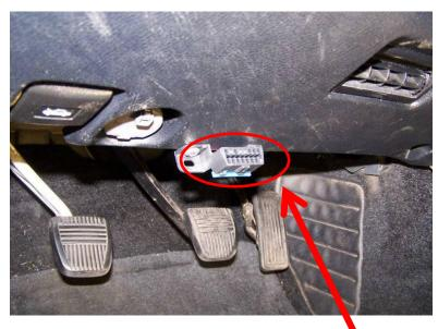
The Male Connector must be inserted into the main vehicle connector you will find under the dash
