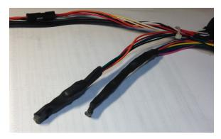
The extra non-essential wires on the LMU's power harness should be individually heat shrunk to avoid accidental contact with other wires or ground.
