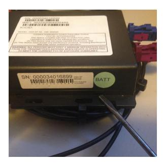
1. If necessary, remove the existing Sim card and insert the new Sim as shown on the photo above.
