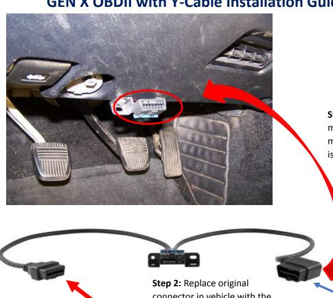
Step 3: The Male Connector must be inserted into the main vehicle connector that is found under the dash
