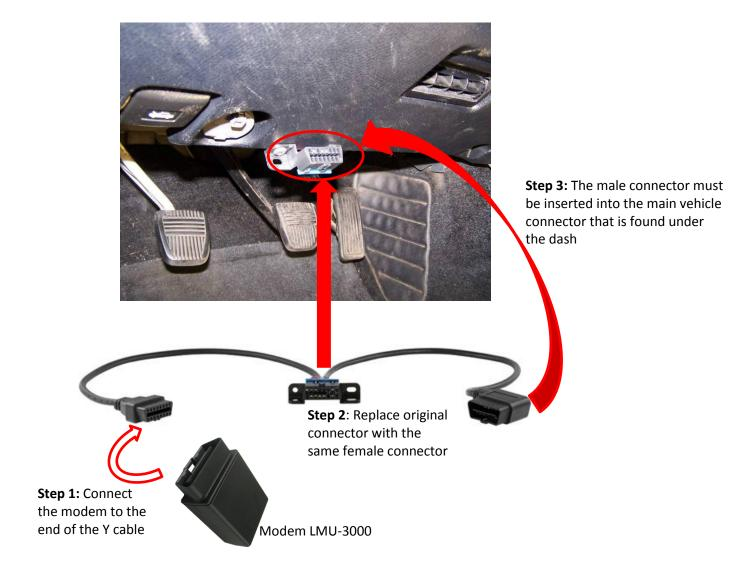
**Note**: If possible, move the modem to the highest point under the dash close to the window. Don't forget to put tie wraps on cables under the dash. Be sure there are no metal obstructions. Plastic material doesn't interfere with cellular and GPS signals. Antennas are built-in for easy installation
